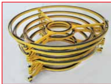
Circular templates for the production of cylindrical cages.
